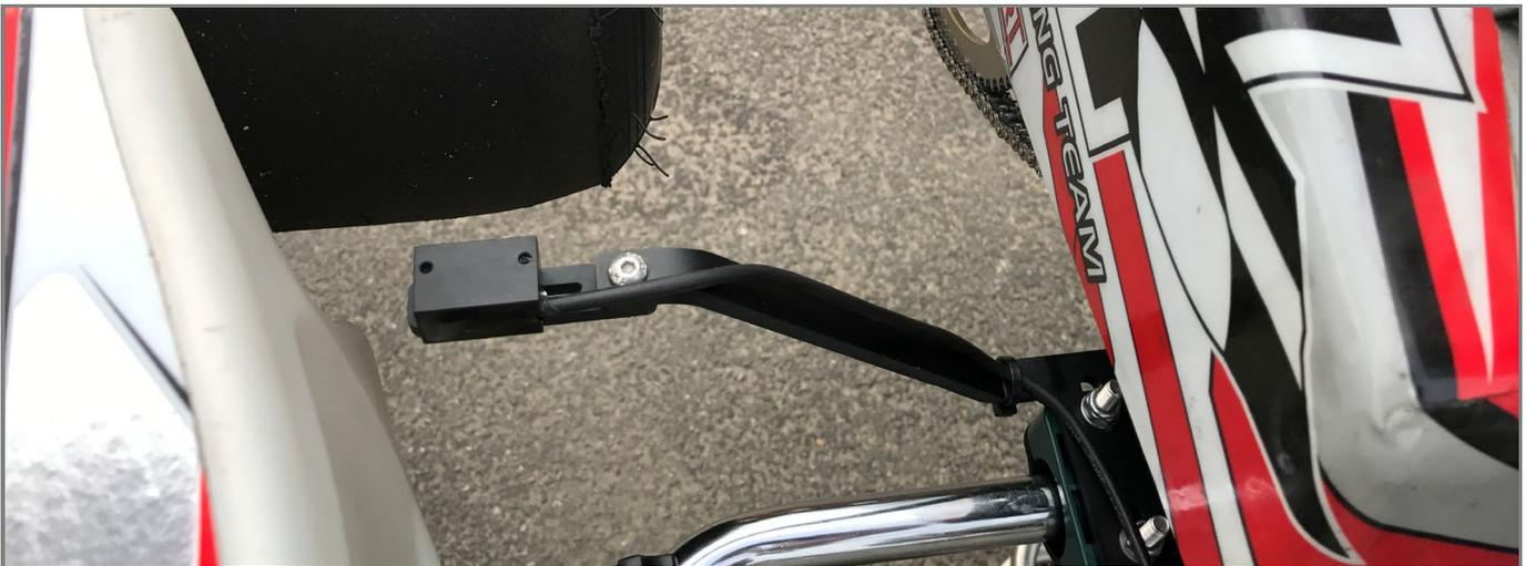
Mounting of brackets for infrared tire temperature sensor - front left tire
